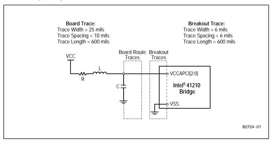
**Note:** Three of these PCI filter circuits must be placed on the system board, one for each of the **VCCAPCI[2:0]** pins on the Intel® 41210 Serial to Parallel PCI Bridge.
